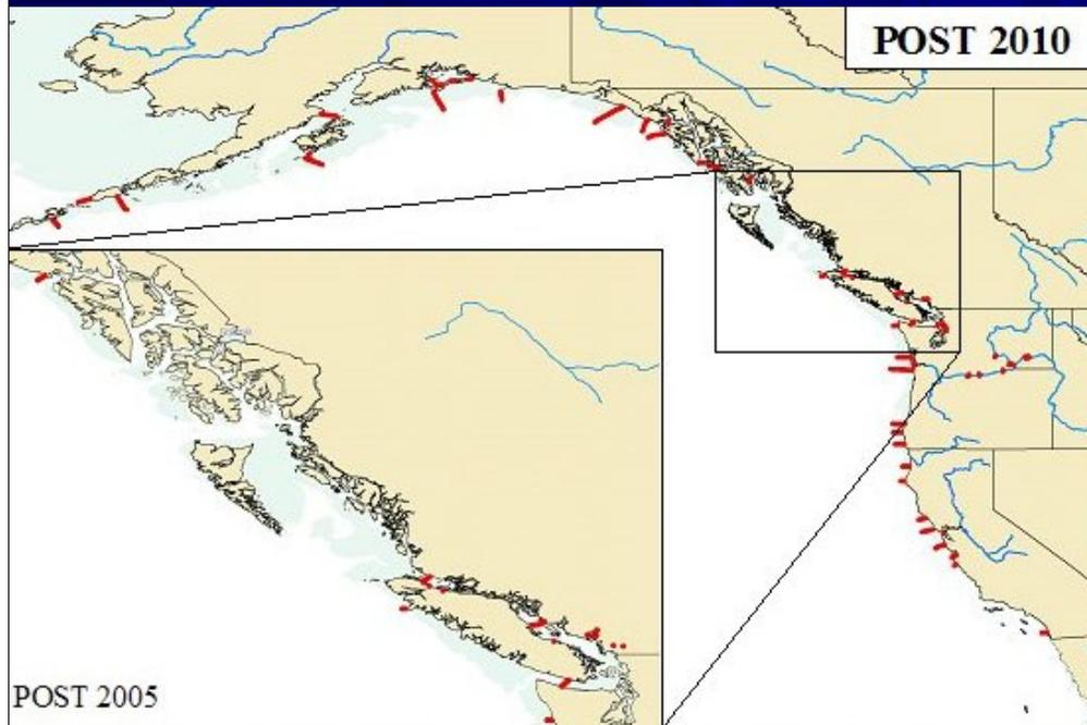
Kintama envisions placement of arrays of acoustic receivers along the continental shelf from California to Alaska. Juvenile salmon equipped with acoustic tags could be traced up or down the coast, and problem areas in the ocean could be identified. For example, if Snake River Chinook migrate to a section of the British Columbia coast where there is an extensive herring fishery, they will lack food and not survive well to adulthood.
